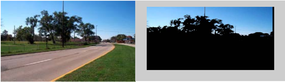
Figure 5: Color-based segmentation using k-means clustering.
